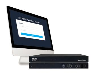
The ZYCOO IAS-L100 is a hardware server preinstalled with the ZYCOO IP Audio Center, providing true out-of-the-box readiness. The IP Audio Center is a comprehensive public address platform offering centralized management of IP audio endpoints.
